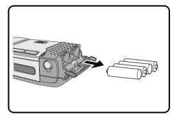
Open the battery cover by performing step 1 of "Loading Batteries" to the left.
